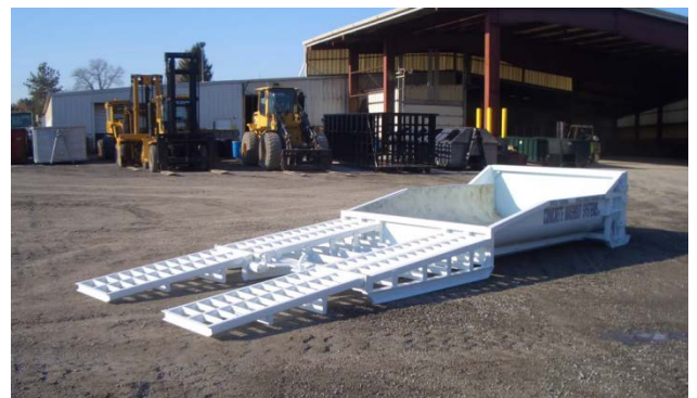
Prefabricated washout container with ramp.
