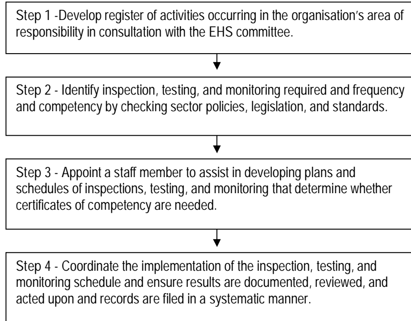
Figure 3-3 Coordinating a Workplace Safety Inspection Schedule
