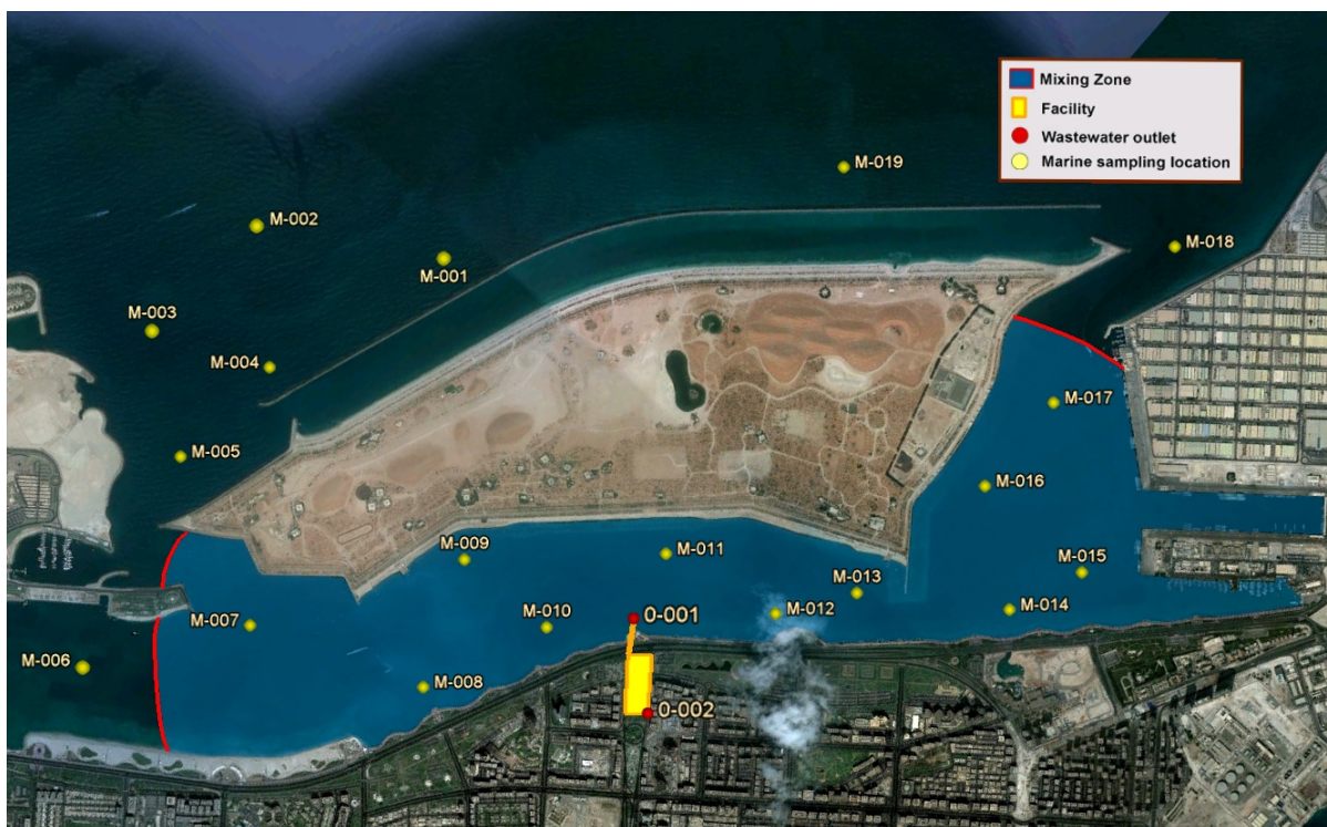
Figure A-1. Example of a map indicating sampling locations for marine water quality measurements.
