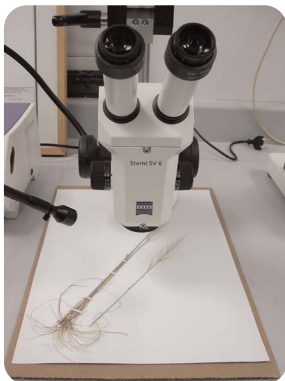
Fig. 10. Close-up of the Zeiss SV6 stereo microscope recently obtained for the ERWDA herbarium.
