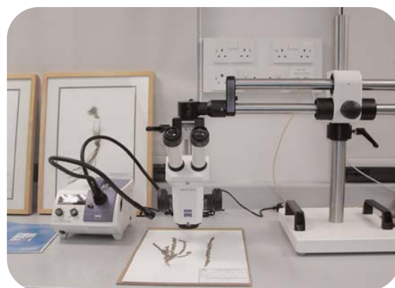
Fig. 9. A stereo microscope is an indispensable piece of equipment for identification purposes. Mounting it on a cross boom allows herbarium sheets to be conveniently examined. The external cold light source (left) provides illumination of a similar spectrum to that of daylight, and does not heat the specimens.
